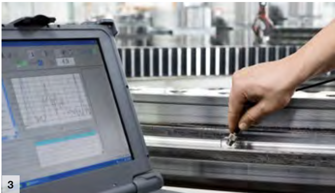
Measurement of hardness depth
