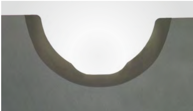
Grinding pattern of a ball bearing slewing ring with hardened case
