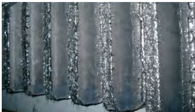
Lubricated gearing in operation
