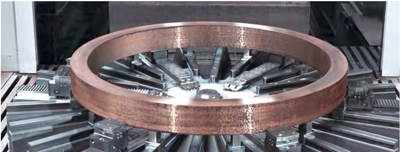
Rolled ring on turning machine
