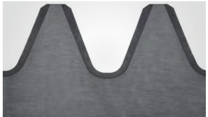
Hardening microsection of tooth spacing hardening
