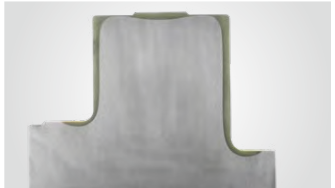
Grinding pattern of a roller bearing slewing ring with hardened case
