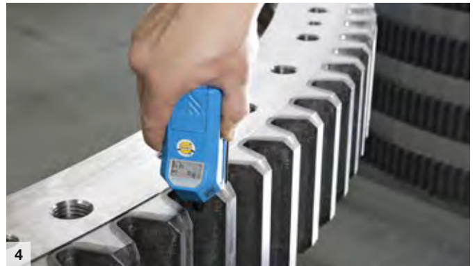
Surface inspection (surface roughness)
