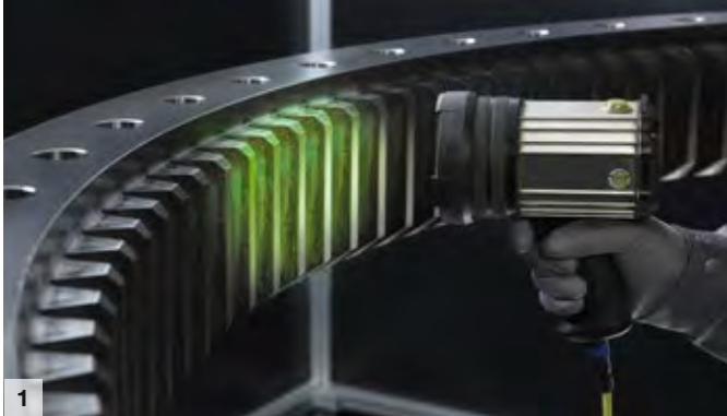
Magnetic particle inspection
