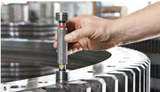
Dimension checks and visual inspection
