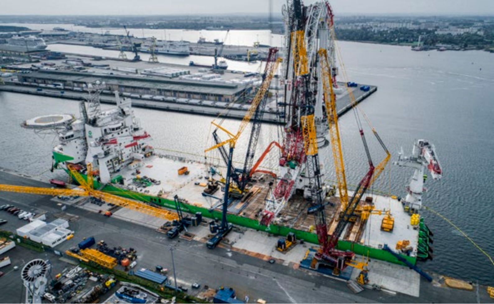
Salvage and dismantling of the HCL 295000 with Liebherr mobile and crawler cranes.
