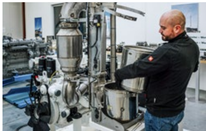
Trainer Thomas Fritsch demonstrates the replacement of a diesel particulate filter on a model at the Liebherr training centre in Ehingen.
